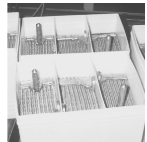
Sandwiches of lead-paste-and-grid form three 2V cells.
